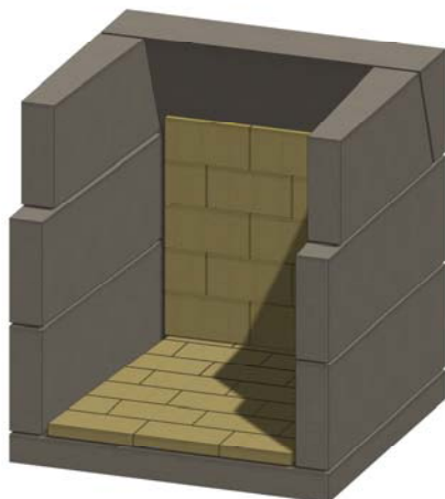
Figure 16. Back Wall Firebrick
